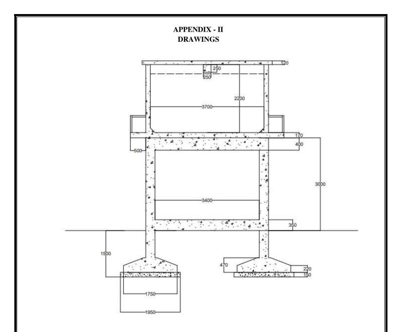
Figure 1. OHSR (All dimensions are in mm)
